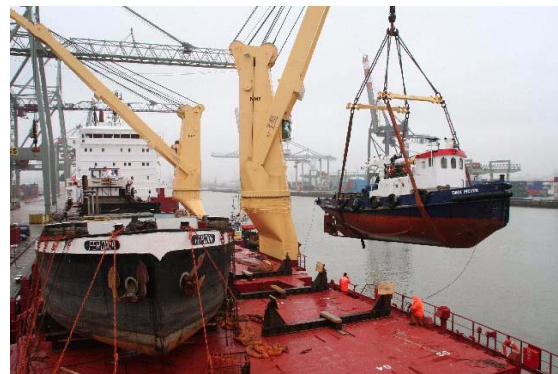
The Dirk Pieter lifted with vessels crane as deck cargo
